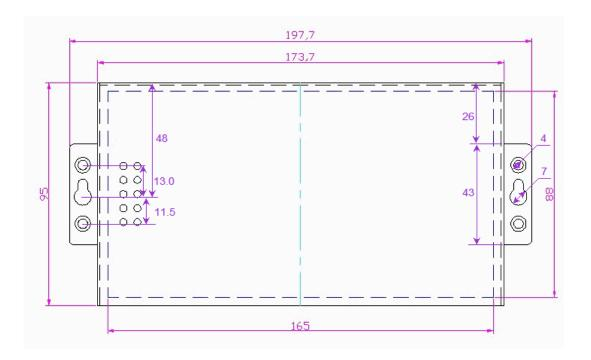
Figure 2 ZLAN5443A Installation Size
