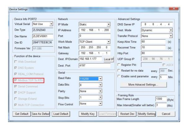
**Figure 6 Modbus Gateway Function Identification**
