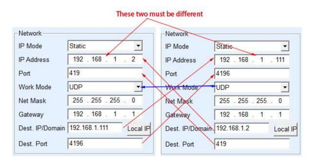
Figure 33 UDP Device Pair-connection Configuration
