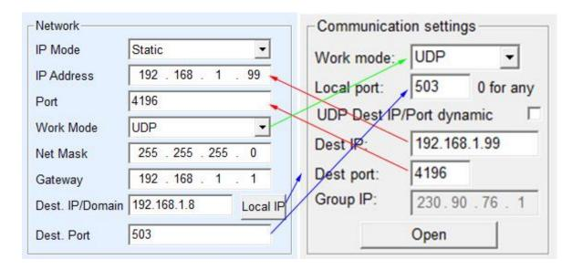
Figure 28 UDP mode Parameter Configuration
