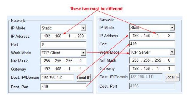
Figure 31 TCP Device Pair-connection Configuration
