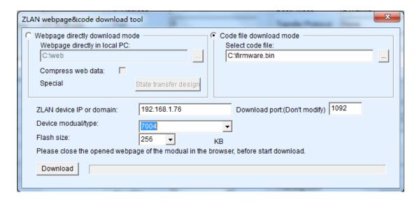
Figure 35 ZLAN7104 Firmware Upgrade Method
